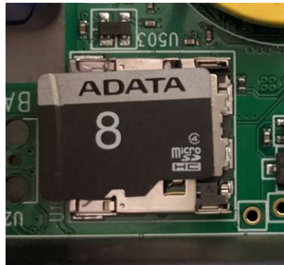
Micro SD card orientation.
